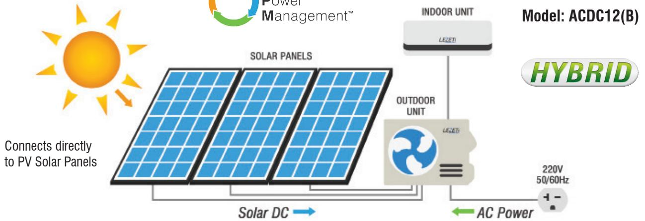
The ACDC12(B) hybrid solar air conditioner runs on DC power directly from solar panels, without needing an inverter, a charge controller, or batteries. The solar DC power directly replaces and significantly reduces the power normally required from the utility grid, cutting daytime energy costs for air conditioning.
